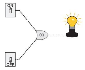
Notice that if we reverse the position of each switch, the light bulb would still remain on. The same is true if both switches are on. However, if both switches were in the off position in this circuit, the light bulb would then turn off.
